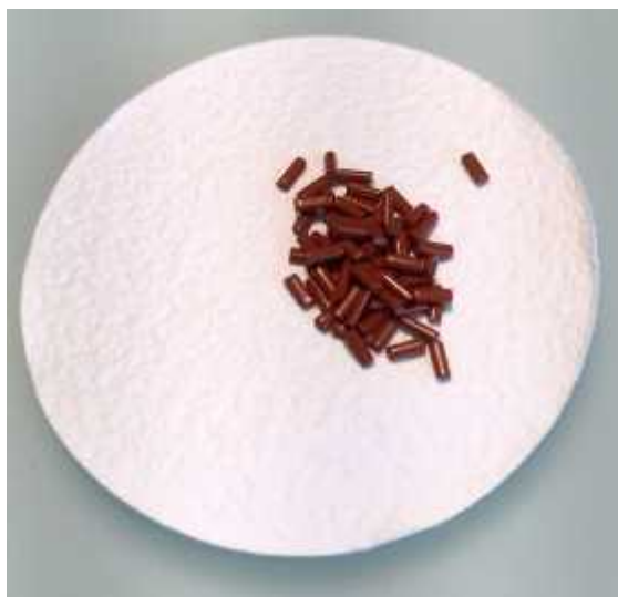
Figure 1 \text{Fe}_2\text{O}_3 /PE rods on a 3 cm diameter filter paper.
